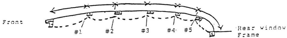
To Measure for the bow spacings - Start at front windshield and measure to the front (face side) of the first bow - Bow #1 face side to #2 bow face side etc. to rear wood frame above the rear window.
